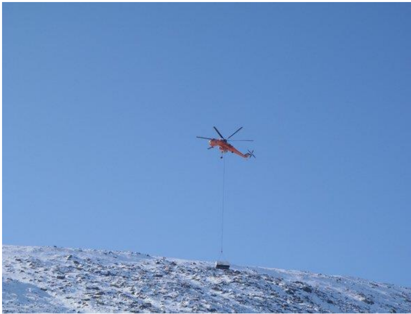
Skycrane helicopter transporting gen-set to Pangnirtung
